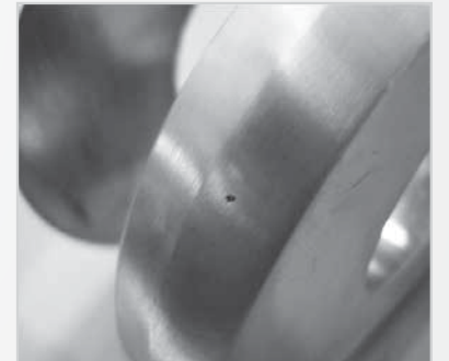
Predicted reoxidation inclusion and corresponding casting defect found in production
