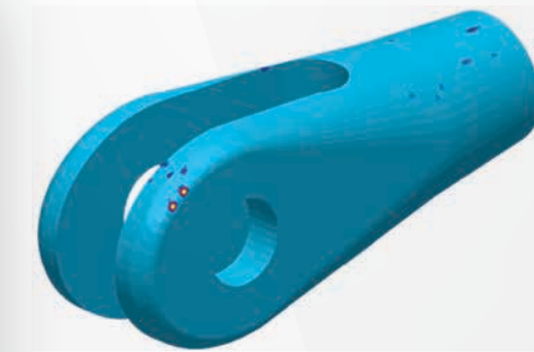
Predicted reoxidation inclusion and corresponding casting defect found in production
