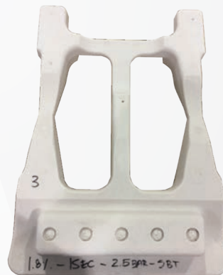
Production core with improved sand compaction and the corresponding sand fraction result after optimizing the tooling
