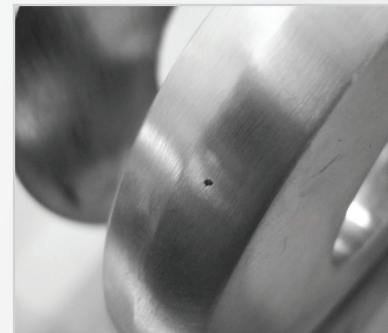
Predicted reoxidation inclusion and corresponding casting defect found in production
